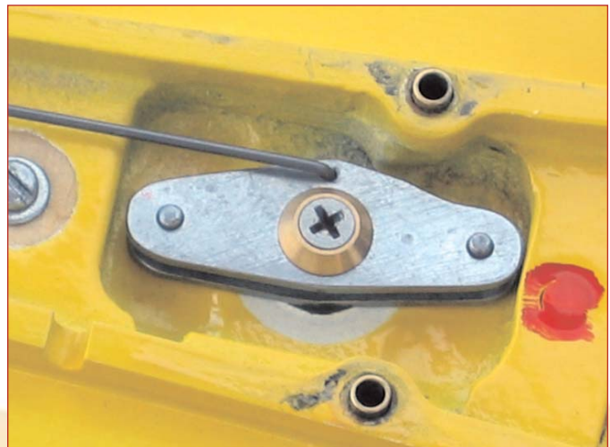
This is how the assembled bell crank looks in the model.
