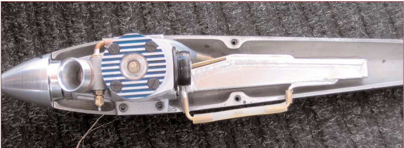
The very clean engine and tank installation are in Jerry Rocha's first-place 21 Sport model.
