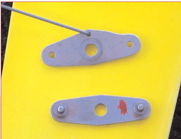
This view of Jerry Rocha's new bell crank shows the two pulleys that the line loops are installed over.
